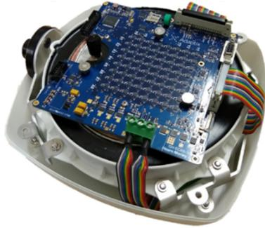
Figure 2: The Adaptix flat panel source array exposed. Courtesy of Adaptix Ltd.
