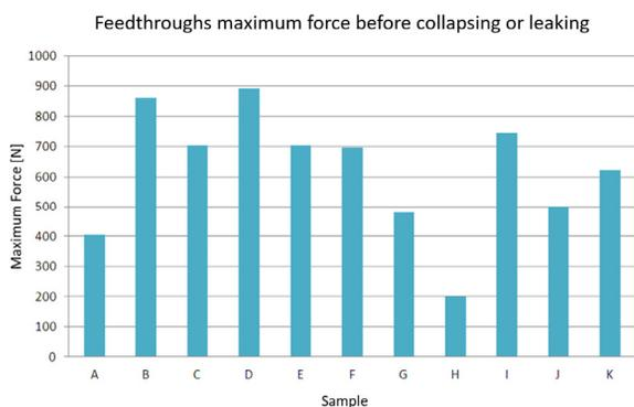
Figure 7: Maximum feedthrough strength results.
