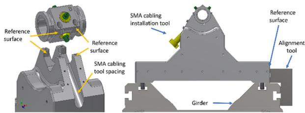
Figure 2: BPM body and support positioning.
