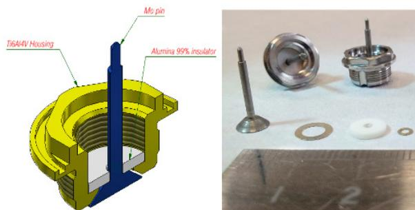
Figure 3: Schematic of feedthrough and its components.
