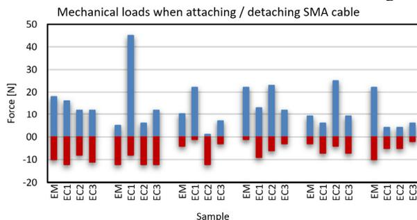
Figure 6: SMA cable mounting loads.
