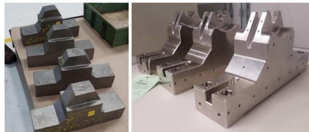
Figure 5: Casted metal and machined supports.
