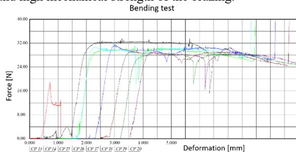
Figure 8: Applied force while bending the pins results.
