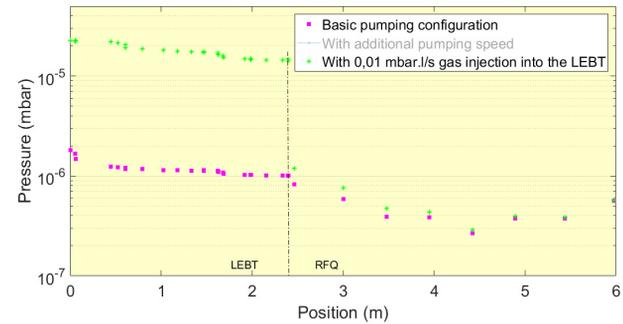
Figure 7: MINERVA LEBT and RFQ pressure tracking after 50 hours pumping.
