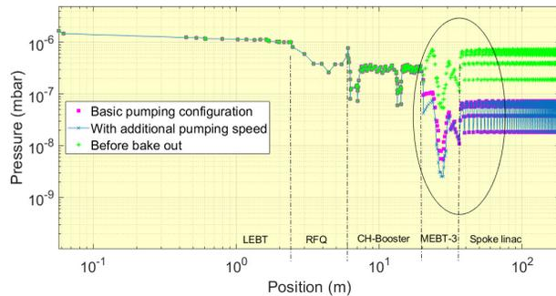
Figure 4: MINERVA pressure tracking after 50 hours pumping at  $T = 293$  K.
