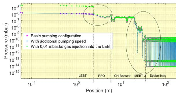
Figure 6: MINERVA pressure tracking after 50 hours pumping at  $T = 2$  K in the linac cavities.
