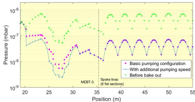
Figure 5: MINERVA MEBT-3 and linac pressure tracking after 50 hours pumping at  $T = 293$  K.
