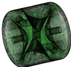
Figure 2: Spoke cavity modelled with Molflow+ software.
