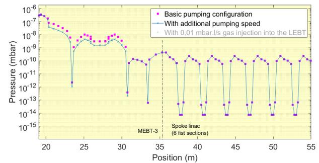
Figure 8: MINERVA MEBT-3 and linac pressure tracking after 50 hours pumping at  $T = 2$  K in cavities.
