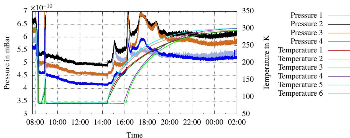
Figure 6: Longtime measurement with both pipes cooled to  $\approx 80$  K. The position of the sensors can be seen in Figs. 4 and 5.
