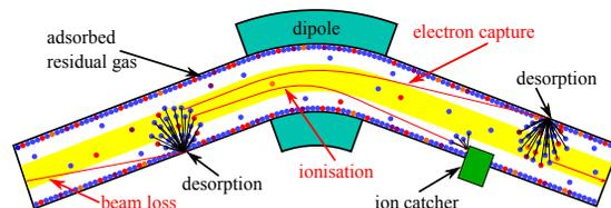
Figure 1: Principle of ionization loss and dynamic vacuum [1].
