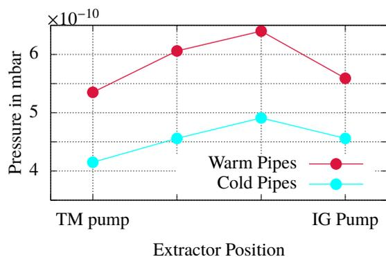
Figure 7: Pressure profile over the chamber, with warm pipes (300 K) and cold pipes (80 K).
