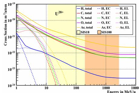
Figure 2: Cross sections for charge exchange for  $U^{28+}$  for different targets, distinguished for electron capture (EC), electron loss (EL) and total cross section. The energy regimes of SIS18 and SIS100 are marked [6].
