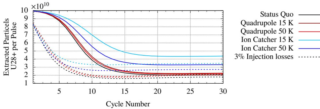
Figure 3: Results from simulations with cryogenic pipes in quadrupole chambers or ion catcher chambers at temperatures of 50 K and 15 K. More parameters are shown in Table 1. Dashed lines show simulations with 3% injection loss, solid lines show the case without injection loss.
