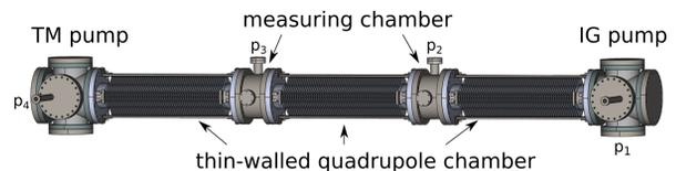
Figure 4: Sketch of the prototype quadrupole chamber with the positions of the pressure sensors  $p_x$ .
