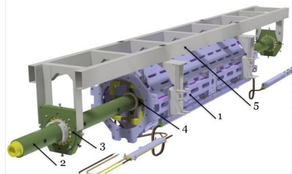
Figure 3: Measuring probe inside the quadrupole magnet: 1 - quadrupole magnet; 2 - probe; 3 - outside self-aligning ceramic ball bearings and adjustable housings; 4 - inside precision ceramic ball bearing with small clearance and tolerances; 5 - frame.
