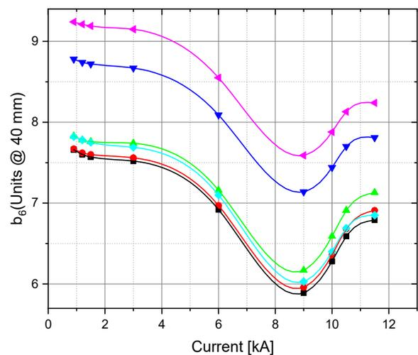
Figure 8: Current dependence of the b6 for series of 6 units (lines are splines).
