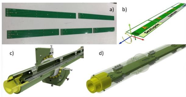
Figure 2: Measuring probe design: a) PCB coils arrays; b) boards arrangement inside unit; c) and d) internal design of the probe.
