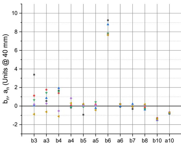
Figure 6: Field quality at 900 A for 6 serial magnets.
