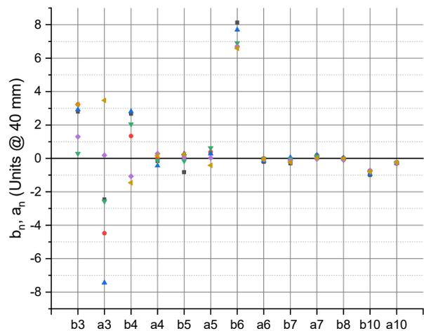
Figure 7: Field quality at 10500 A for 6 serial magnets.
