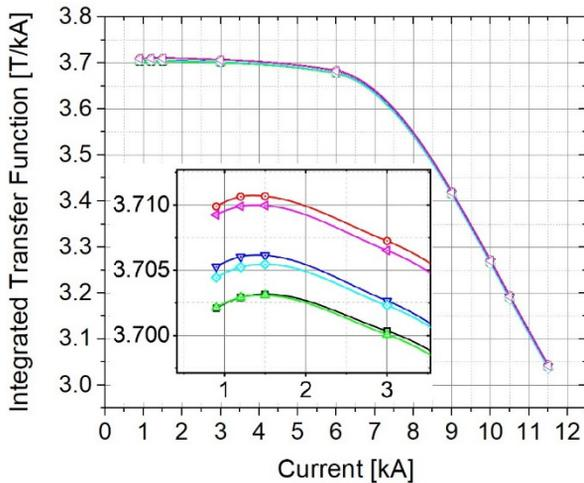
Figure 5: Current dependence of the integrated transfer function for series of 6 units.
