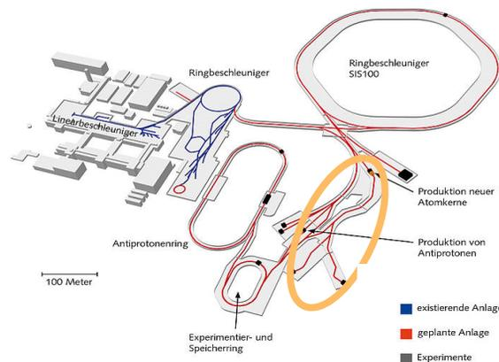
Figure 1: Layout of FAIR. On the left is the existing GSI, the position of Super-FRS with its different branched is indicated by the orange circle.
