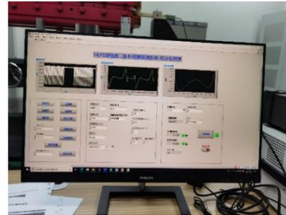
Figure 4: Interface of the translation long coil uniformity measurement program.
