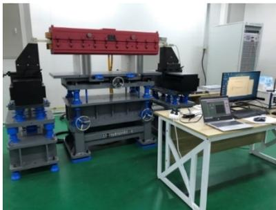
Figure 3: The long coil dynamic measurement system for dipole magnets of HEPS Booster.
