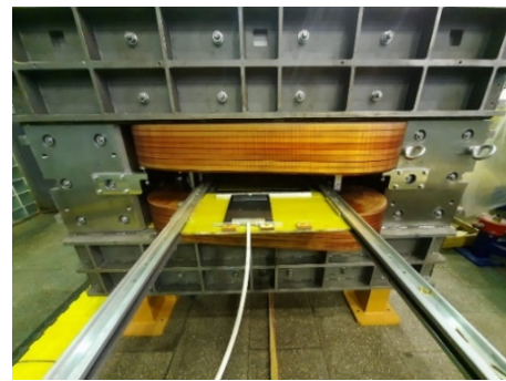
Figure 6: CR dipole precision measurement system based on carriage with Hall sensors, plate and rail.
