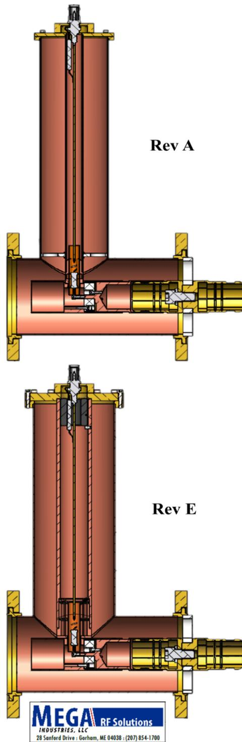
Figure 2: Comparison of cross-sections for Mega Revision A and Revision E tees.
