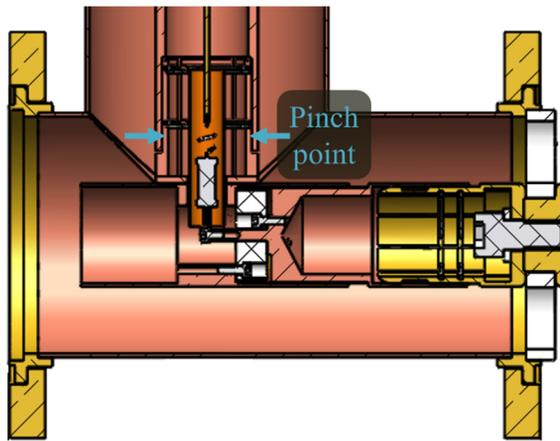
Figure 3: Pinch point on bias tee stub connector.
