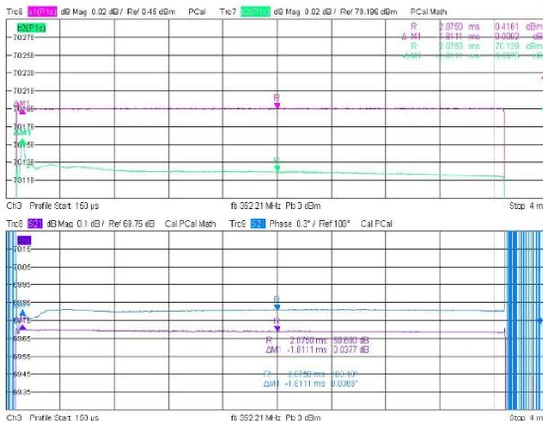
Figure 3: 10 kW Driver RF pulse amplitude (Trc 6) and phase (Trc 8) compared with the driving signal (Trc 7 and Trc 9). RF overshooting has been mitigated by modulating the drain voltage 200  $\mu$ s before the RF pulse start.
