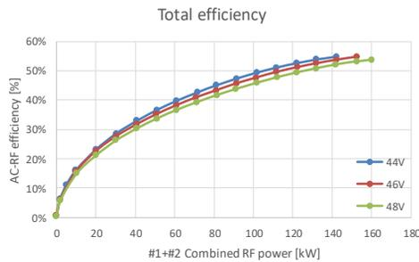
Figure 5: the AC-RF conversion efficiency as a function of output RF power in different DC voltage settings for 2-way combination of 80 kW SSPAs.
