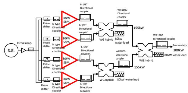
Figure 1: The topology of 300 kW fully solid-state transmitter.
