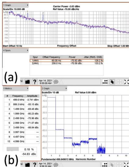
Figure 6: The quality of the combined RF of 2 80kW SSPA towers: (a) phase noise: -70.92 dBc@60Hz, -70.58 dBc@260Hz (b) harmonics: -55.15 dBc@2<sup>nd</sup> and -69.48 dBc@3<sup>rd</sup> harmonic.
