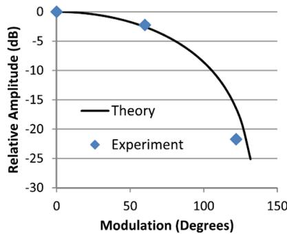
Figure 2: Power at fundamental frequency as function of driver phase modulation.
