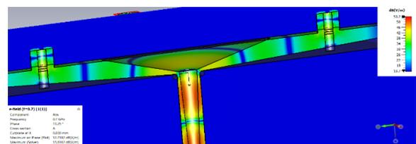
Figure 9: High Frequency Structure Simulation of input coupler for multiple beam IOT.
