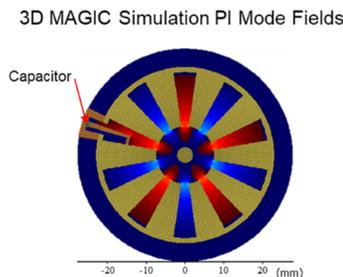
Figure 3: 3D MAGIC simulation of pi mode fields in a magnetron where varactors modulate capacitance of a cavity.
