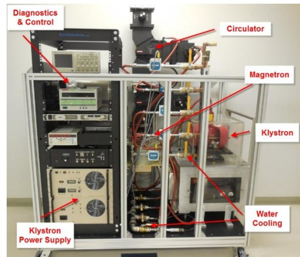
Figure 1: 1.3 GHz, 100 KW, Magnetron System with fast phase and amplitude control.
