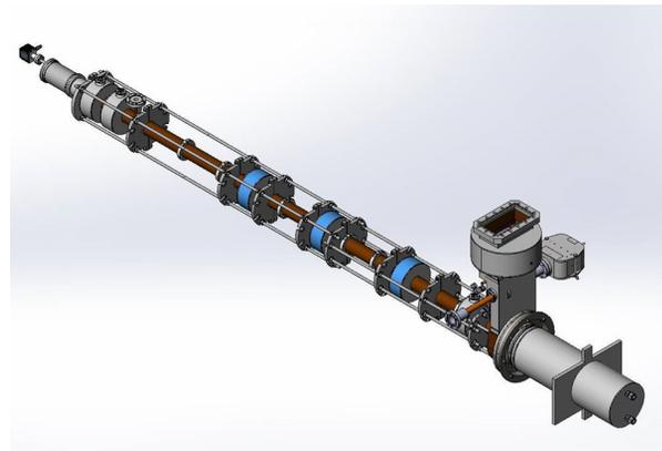
Figure 5: Solid model of 1.3 GHz klystron designed to produce 100 kW at more than 80% efficiency.
