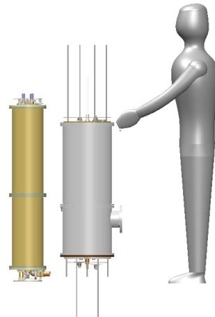
Figure 8: 350 MHz, 200 kW RF system source.
