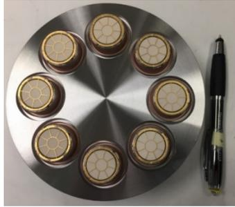
Figure 6: Array of eight grid-cathode assemblies to produce 230 kW of beam power.
