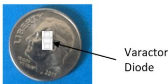
Figure 4: Microsemi GC1712 varactor diode.
