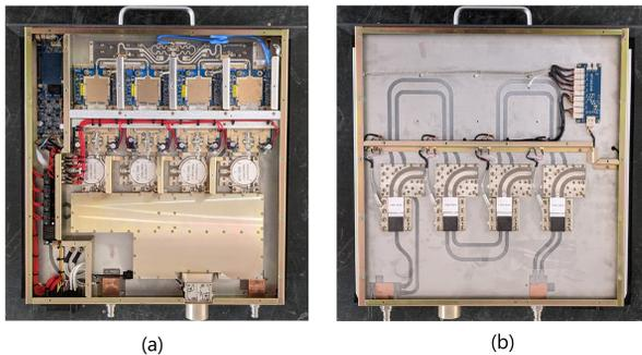
Figure 2: The 2-kW amplifier module: (a) front side view and (b) back side view.
