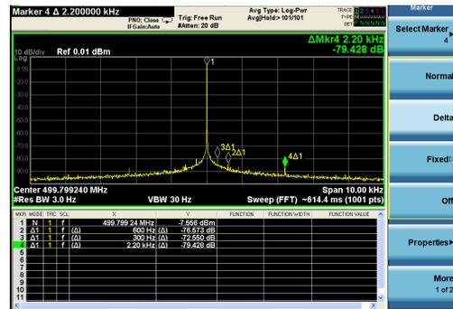
Figure 7: Spurious of the 22-kW amplifier cabinet.
