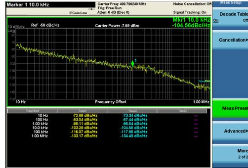
Figure 8: Phase noise of the 22-kW amplifier cabinet.
