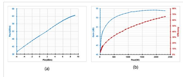
Figure 3: Measurement results of the 2-kW amplifier module: (a) output power vs. input power and (b) gain and DC to RF efficiency vs. output power.
