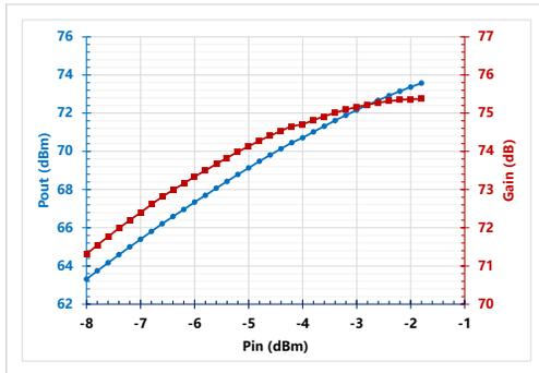
Figure 5: Measurement results of the 22-kW amplifier cabinet: output power and gain vs. input power.
