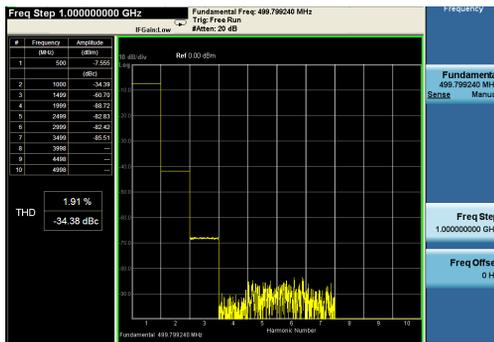
Figure 6: Harmonic of the 22-kW amplifier cabinet.
