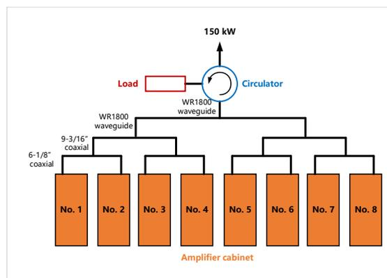
Figure 1: The diagram of combining route of the 500-MHz 150-kW SSA.
