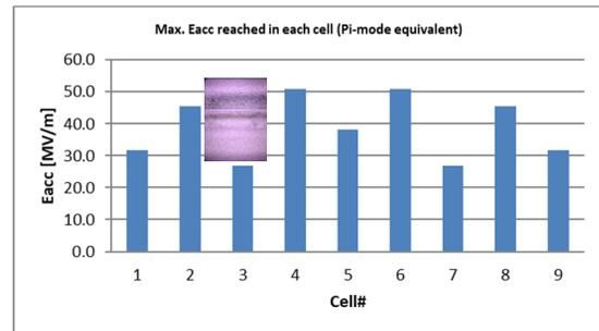
Figure 7: Gradient capability of each cell of LSF9-1. Inset shows the RF surface image of quench location in Cell#3.
