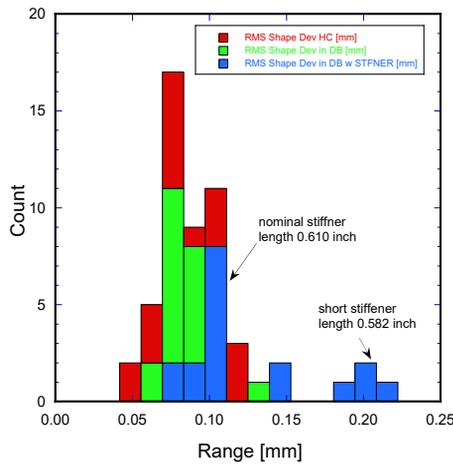
Figure 2. Half-cell shape accuracy statistics.
