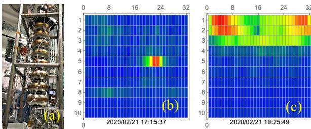
Figure 5: 1622 sensors attached to LSF9-1 (a) and X-ray hot spots captured by Kyoto U sX-mapping system (b, c).
