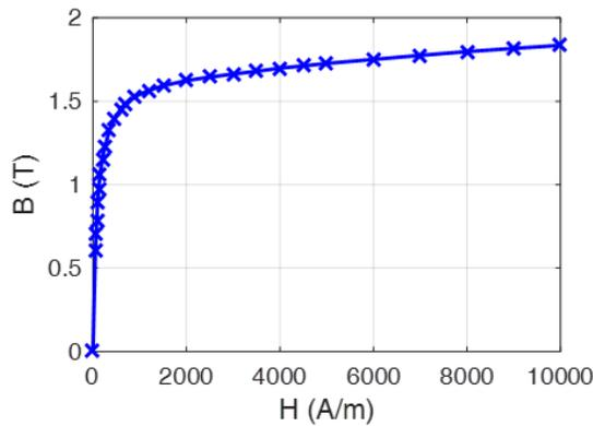
Figure 6: The B-H curve of DT4.
