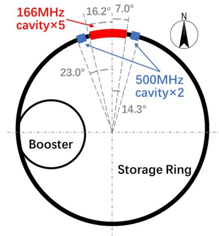
Figure 1: Locations of SC cavities in HEPS storage ring.
