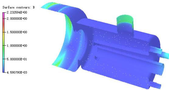
Figure 4: Residual magnetic field on the 166 MHz cavity wall (Unit: Gs).
