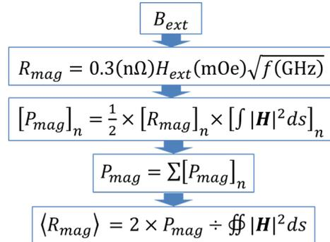
Figure 5: Calculate the equivalent residual resistance according to the external magnetic field.
