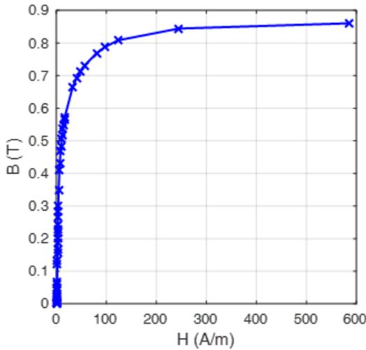
Figure 3: The B-H curve of 1J79 in liquid helium temperature.
