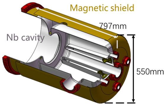
Figure 2: 166 MHz SC cavity magnetic shielding structure.
