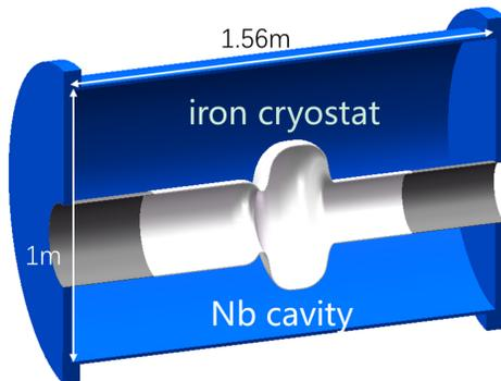
Figure 7: Simplified 500 MHz SC cavity magnetic shielding model.
