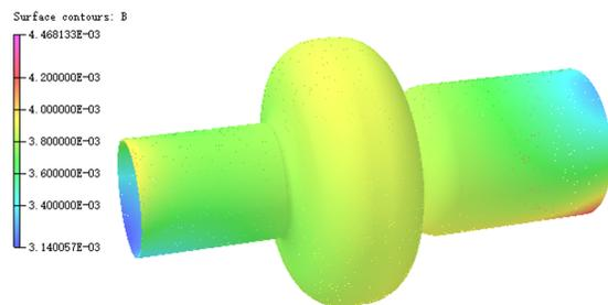
Figure 8: Residual magnetic field on the 500 MHz cavity wall (unit: Gs).
