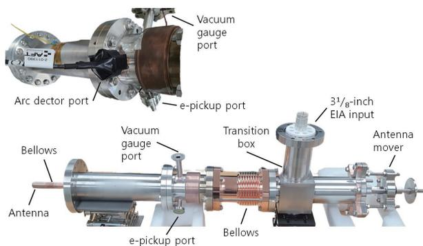
Figure 1: Manufactured model of the 325 MHz power coupler.
