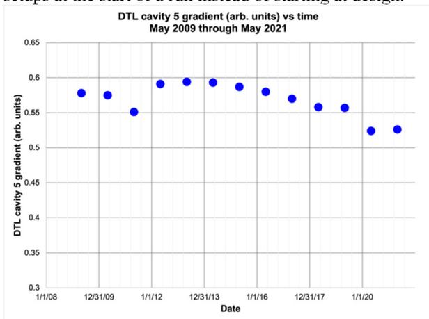
Figure 3: DTL cavity 5 field setting over time. Before 2015 the field was set using PASTA. Once the method was switched to pattern based 360-degree scan setup it enabled the ability to move the field setting away from design and set it based for minimum fault rate. The continual decrease in field may indicate a developing issue with the DTL5 cavity.
