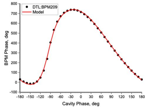
Figure 5: Example of a DTL cavity 2 phase scan showing the model (red line) and the BPM data (black points).
