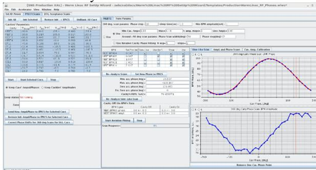
Figure 4: Warm linac tuner wizard window showing a MEBT cavity scan. The top plot on the right shows the BPM phase as a function of the RF cavity phase. The lower plot is the beam current seen by the BPM used during the scan.
