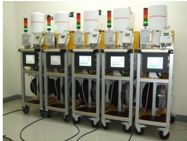
Figure 3: Real-time radiation monitoring stations with interlock.
