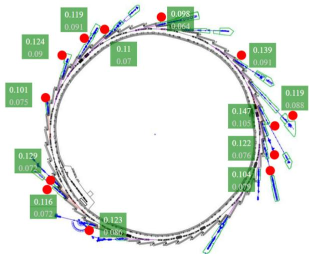
Figure 4: Positioning of monitors for TPS beamlines.
