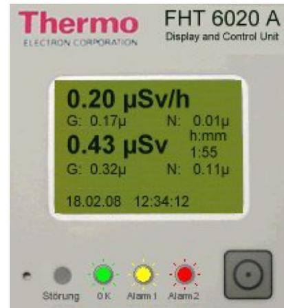
Figure 6: Display of Thermo FHT 6020 controller.
