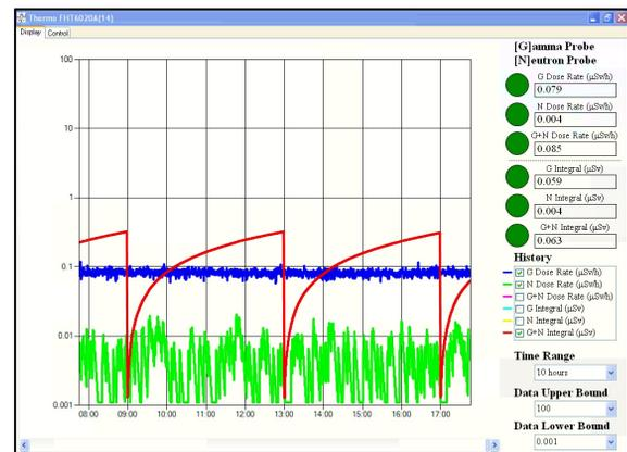
Figure 7: Local display interface of radiation data.
