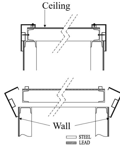
Figure 9: Side view of ceiling quick-release parts.
