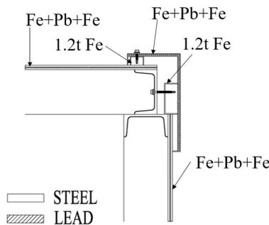
Figure 7: structure of the roof joints outside the hutch.
