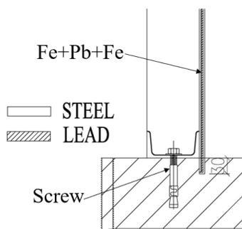
Figure 8: ground-entry type, to prevent radiation leakage.
