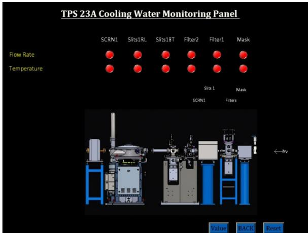
Figure 8: The picture of Cooling Water Monitoring Panel.
