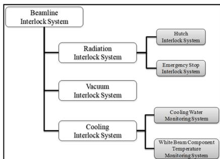
Figure 1: System architecture of Beamline Interlock System.
