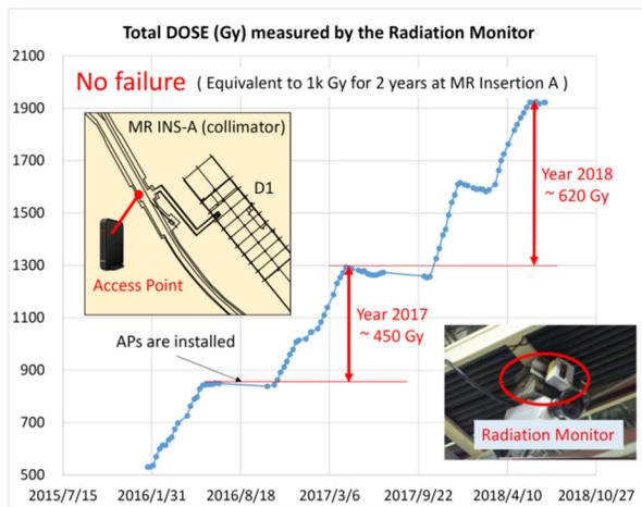
Figure 2: Radiation tests in J-PARC MR.
