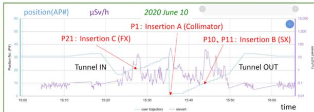
Figure 5: A demonstration of going around the MR tunnel with the smartphone connecting the radiation counter.
