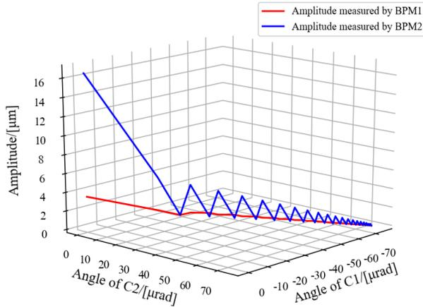
Figure 3: Changes of beam position amplitude in two-to-two correction adjustment.
