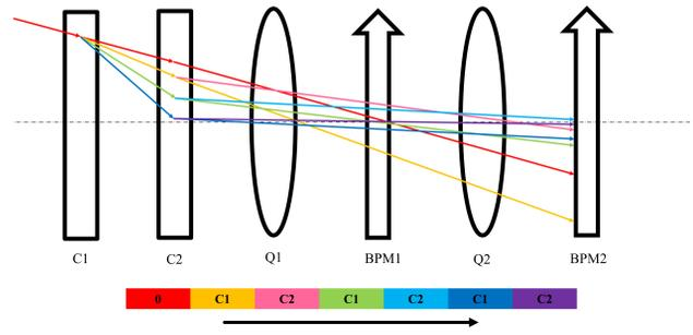
Figure 5: Changes of beam orbit during the correction process. The arrows indicate the order of corrections and the word corresponding to the color indicates the corrector which is adjusted in corresponding correction.
