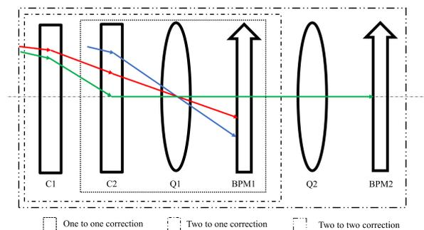
Figure 2: Schematic diagram of the three arrangements. The blue line represents the beam orbit after one-to-one correction, the red line represents the possible beam orbit after two-to-one correction, and the green line represents the target beam orbit.
