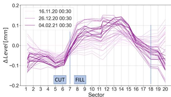
Figure 5: Vertical deformations acquired by the HLS from Nov./2020 to Apr./2021.
