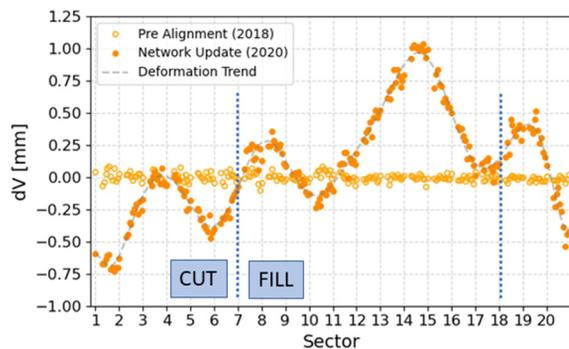
Figure 4: Vertical absolute position of SR magnets after the course alignment (2018) and during the network update (2020).
