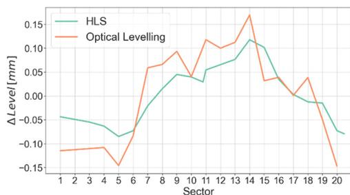
Figure 2: Comparison of the deformation indicated by the HLS and the one measured by Optical Levelling.
