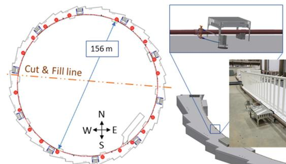
Figure 1: HLS's layout and assembly details. Red dots and lines represent the sensors and pipe network, respectively.
