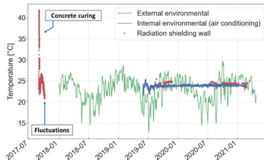
Figure 7: Timeseries of environmental and structural temperatures. Courtesy: Center for Meteorological and Climate Research Applied to Agriculture (CEPAGRI).
