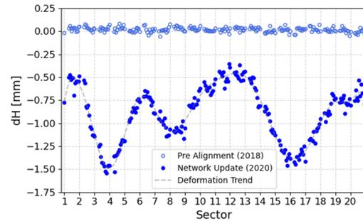
Figure 6: Horizontal absolute position of SR magnets after the pre alignment (2018) and during the network update (2020).
