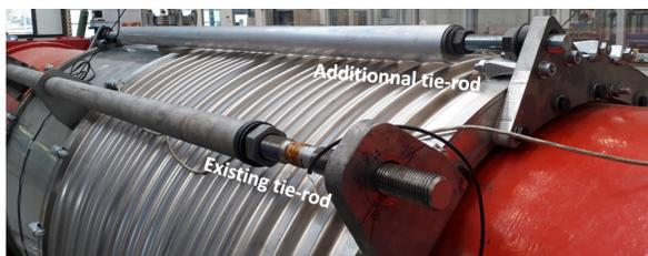
Figure 7: Prototype of additional tie-rod (autumn 2019).
