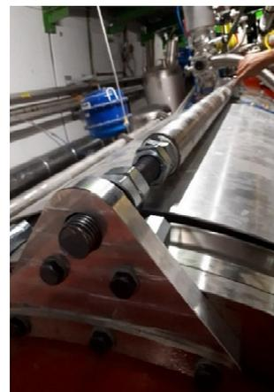
Figure 8: Additional tie-rod implementation in the LHC.
