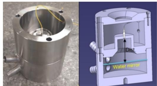
Figure 5: FSI-HLS sensor and its operation principle.
