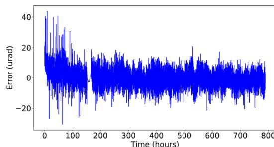
Figure 8: Error between the FSI inclinometer and Sherborne LSOC-1 inclinometer.
