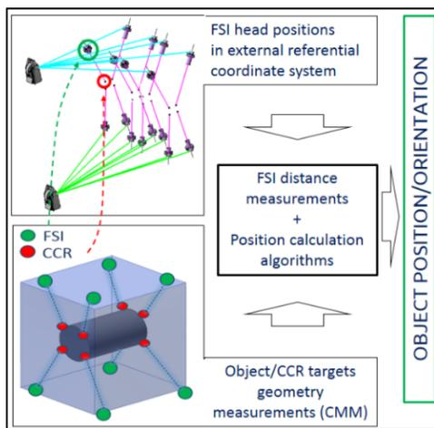
Figure 3: Sequence of measurements for intra-cryostat position monitoring.
