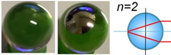
Figure 2: Glass ball reflector (uncoated, coated, principle).
