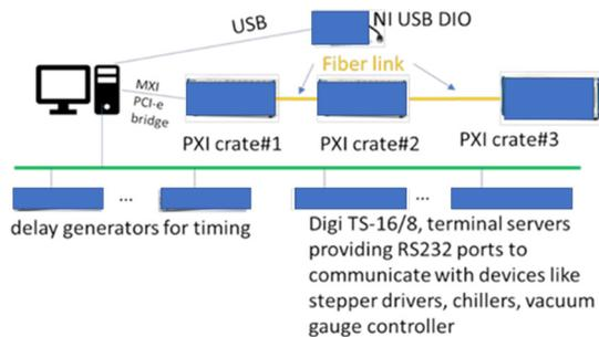
Figure 2: Hardware directly connected to control PC.
