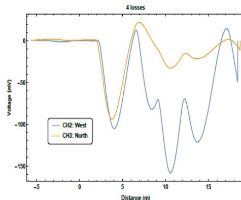
Figure 3: Variation in the signal generated by OBLMS for varying beam charges at four different loss locations simultaneously placed in the CLARA front end.
