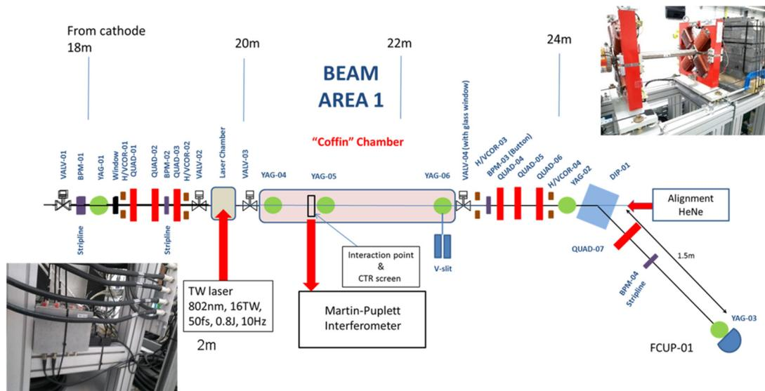
Figure 1: Two fibres of oBLMS on the CLARA beam area 1. The schematic in the middle is the beamline where two fibres are installed parallel to one another. The photograph (inset left) shows the sensor unit/fibre coupling and the photograph (inset right) shows the fibre location along the beam line (black cables near the bottom of the red quadrupole magnets).
