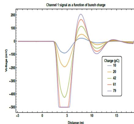
Figure 2: Variation in the signal generated by an oBLM for varying beam charges at one loss location in the CLARA front end.
