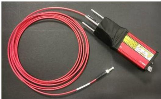
Figure 4: ns-pulsed laser prototype for online testing and calibration of the OBLMS system.
