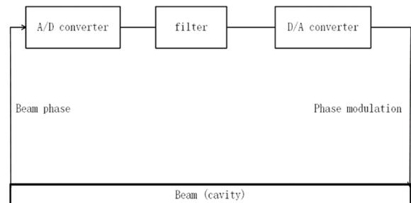
Figure 4: The schematic of the optimized phase loop in the RF system of the RCS.
