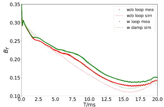
Figure 3: The left shows the measured beam phase with and without the designed phase loop. The right shows the bunch factor with and without the loop: measurement and simulation.
