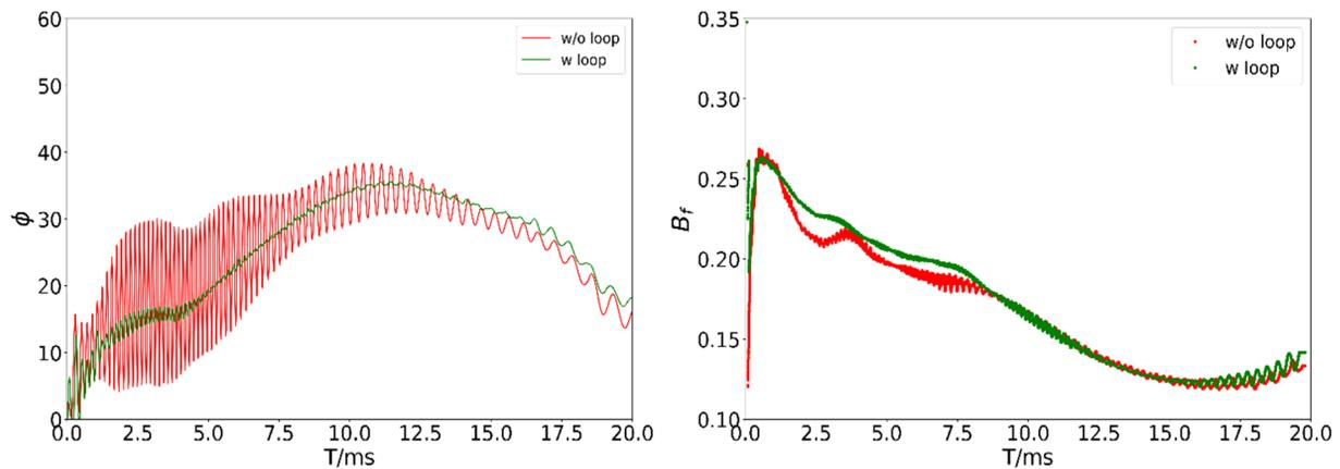
Figure 5: The measured beam phase (left) and the bunch factor (right) with and without the optimized phase loop. The measured signal and data processing give the bunch factor difference before 8 ms in the right.
