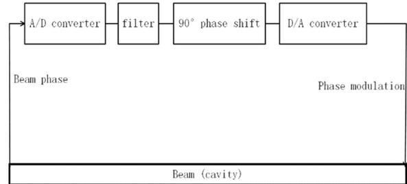
Figure 2: The schematic of the designed phase loop in the RF system of the RCS.
