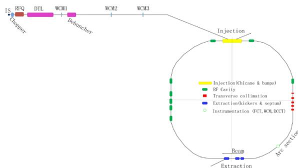
Figure 1: The layout of CSNS accelerator: linac and RCS.
