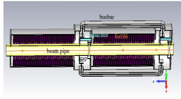
Figure 3: The CST simulation mode of the cavity.
