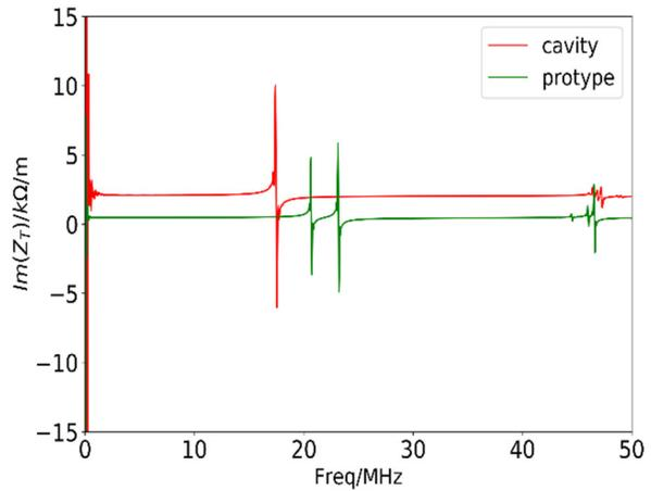
Figure 4: The transverse impedance of the ferrite cavity.
