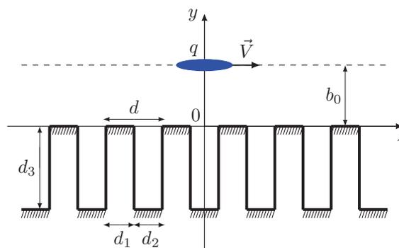
Figure 1: The corrugated structure and the moving bunch.
