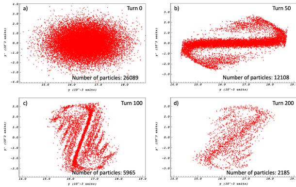
Figure 3: Phase space when a quadrupole perturbation is applied to the T-insert lattice, at a frequency of  $2 \cdot 2\pi Q$ , with the octupole potential switched off.
