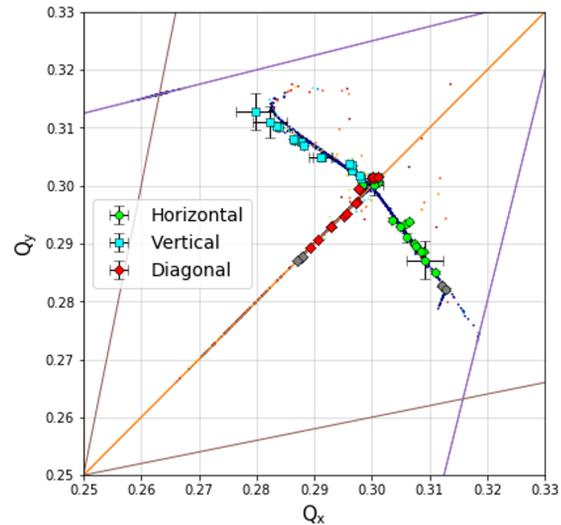
Figure 2: QI tune map at nominal  $1.0\ \text{A}$  current overlaid with FMA simulation (dark blue). Gray markers indicate significant but not total beam losses.
