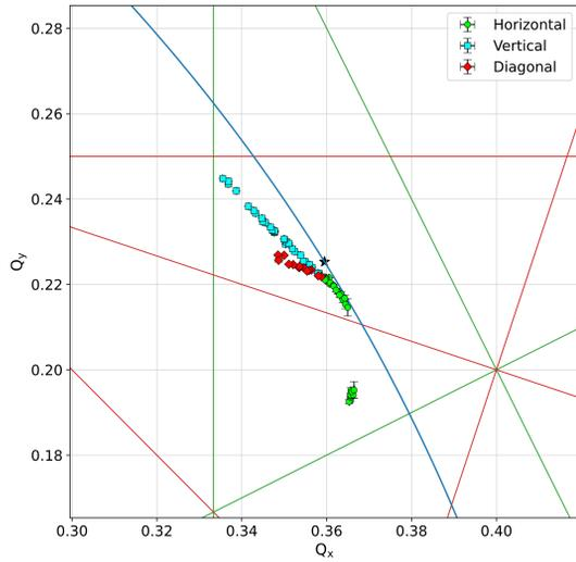
Figure 3: DN tune map at  $t = 0.218$ . Theoretical small amplitude tune is denoted with a black star.
