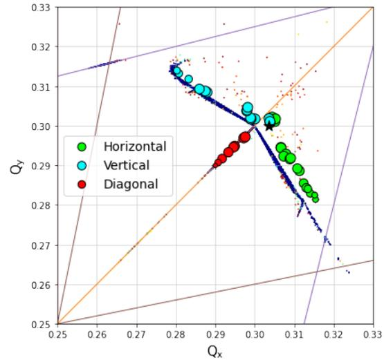
Figure 4: QI tune map at nominal 1.0A current and working point error of  $\Delta Q_x = +0.003$ , overlaid with nominal FMA simulation. Decreasing marker size denotes beam losses.
