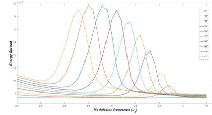
Figure 3: Energy spread vs. the modulation frequency. The difference color curves represent the different modulation amplitude.
