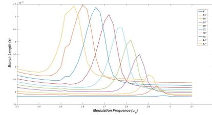
Figure 2: Bunch length vs. the modulation frequency. The difference color curves represent the different modulation amplitude.
