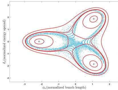
Figure 1: Comparison between particles distribution and K-constant contours. The blue points represent particles in normalized phase space, and the red curves are the K-constant contours in different Hamiltonian, and the asterisks represent the results of SFPs calculated by theoretical model.
