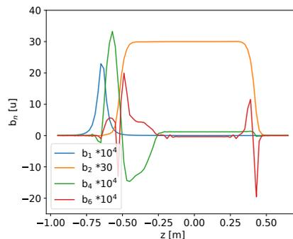
Figure 4: Longitudinal profile of the harmonics in the  $Q_3$  magnet from the Left side of IP5.
