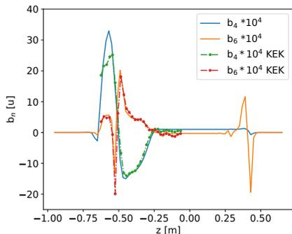
Figure 3: Comparison between the harmonics longitudinal profile of the Roxie 3D machine-like model and the longitudinal magnetic measurements performed at KEK. Courtesy of H. Nakamoto (KEK).
