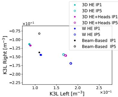
Figure 6: Integrated strength of the  $b_4$  corrector computed for different models in IR1 and IR5, and 60 slightly different  $b_2$  values.
