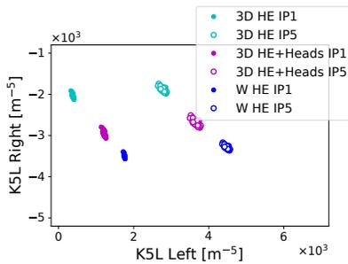
Figure 7: Integrated strength of the  $b_6$  corrector computed for different models in IR1 and IR5, and 60 slightly different  $b_2$  values.
