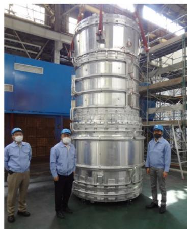
Figure 5: Cold mass of the capture solenoid magnet.
