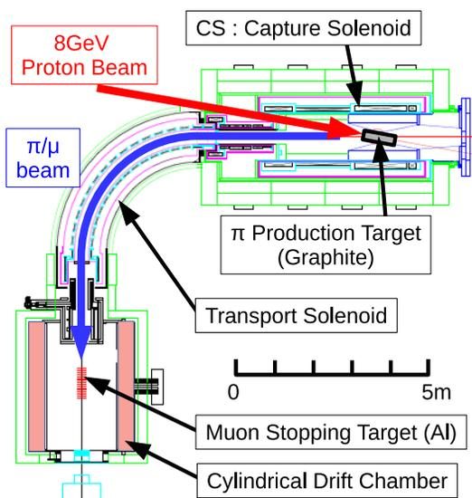
Figure 1: The COMET experiment setup at Phase-1.
