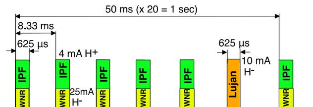
Figure 4: Layout of Lujan/WNR/IPF beams. Beams delivered to pRad or UCN facilities, “steal” their time cycles from WNR beam.
