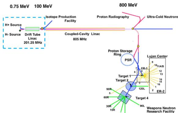
Figure 1: Overview of the existing LANSCE accelerator and user facility complex.
