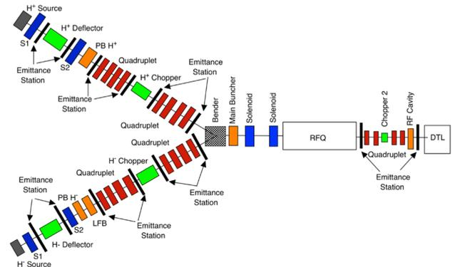
Figure 5: Layout of the new RFQ - based 3-MeV injector.
