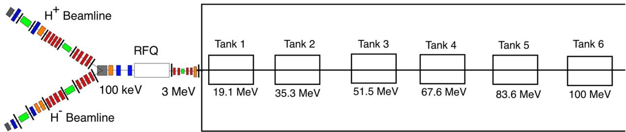
Figure 2: Layout of the new 100 MeV LANCE Front End Accelerator Facility.
