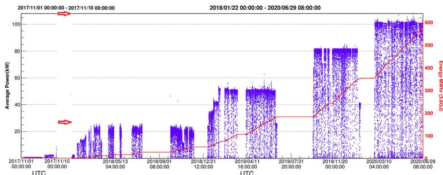
Figure 1: Beam power ramp-up history of CSNS/RCS, where the blue bars correspond to the beam power, while the red line shows the accumulated beam power.
