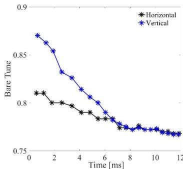
Figure 6: The measured tune variations during acceleration.
