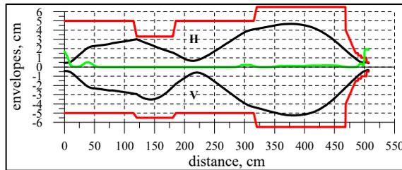
Figure 7: Horizontal (H) and vertical (V)  $^{197}\text{Au}^{26+}$  beam envelopes, aperture (red line) and longitudinal magnetic field (green line).
