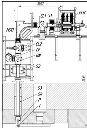
Figure 2: Scheme of the axial injection beam line.
