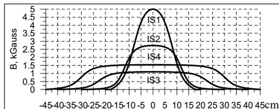
Figure 3: On-axis magnetic field of solenoids.
