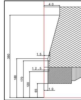
Figure 4: Magnetic plug scheme.
