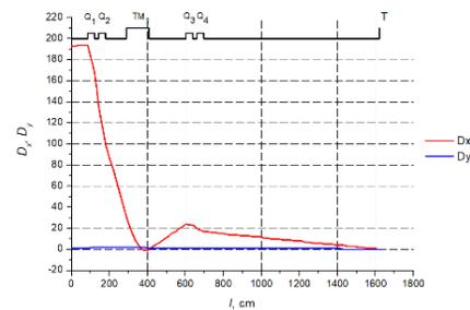
Figure 4: Horizontal dispersion function  $D_x$  (red curve) and vertical dispersion function  $D_y$  (blue curve) of the ion beam 209Bi38+.
