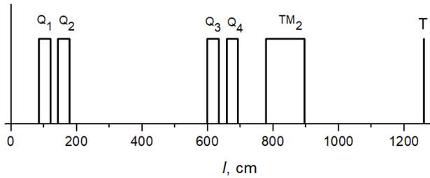
Figure 5: Scheme of the beam line #2. Here Q1-4 are quadrupoles, TM2 is the bending magnet, T is a target.
