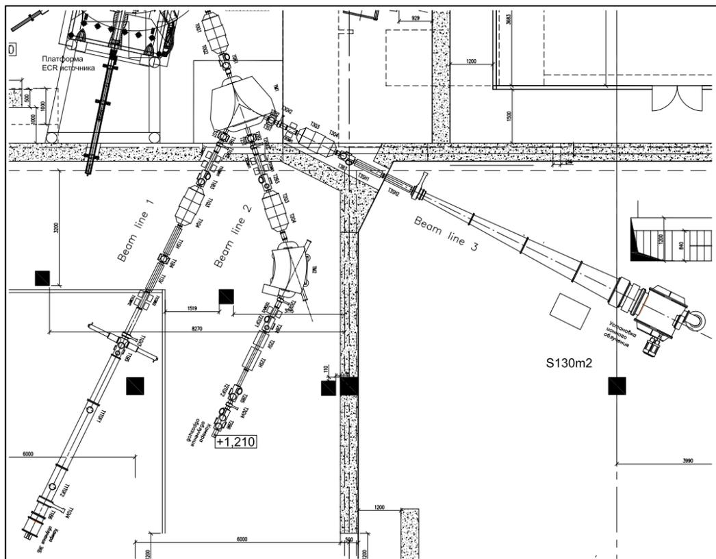
Figure 1: Layout of the beam lines for heavy ion transportation.
