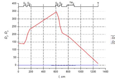
Figure 7: Horizontal dispersion function  $D_x$  (red curve) and vertical dispersion function  $D_y$  (blue curve) of the ion beam  $^{197}\text{Au}^{26+}$ .
