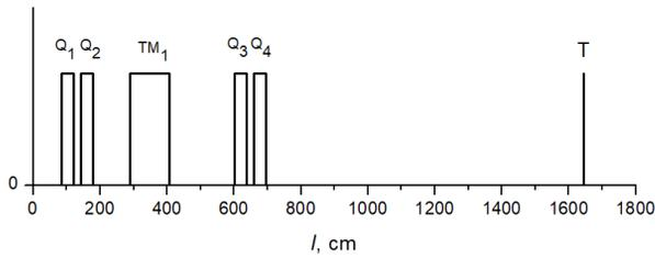
Figure 2: New scheme of the beam line #1. Here Q1-4 are quadrupoles, TM1 is the bending magnet, T is a target.
