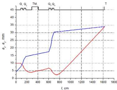
Figure 3 : Horizontal (red curve) and vertical (blue curve) envelopes of the ion beam 209Bi38+.
