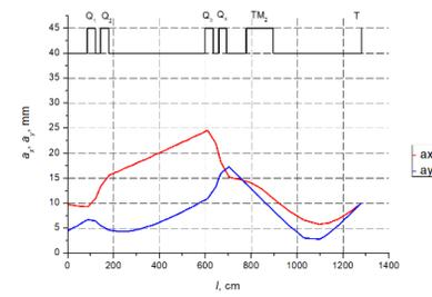
Figure 6: Horizontal (red curve) and vertical (blue curve) envelopes of the ion beam  $^{197}\text{Au}^{26+}$ .
