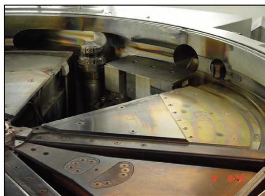
Figure 1: The groove in the long pole, the gradient corrector and the beam separator in the prototype.
