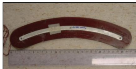
Figure 5: Harmonic coil in the prototype.
