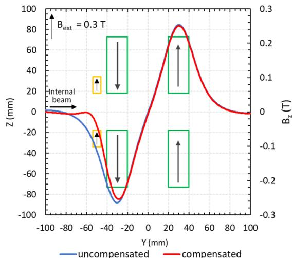
Figure 3: Schematic cross section of the gradient corrector. The shape of the produced magnetic field is also showed together with the two small compensating blocks.
