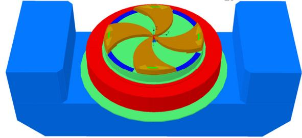
Figure 5: Computer model of U400M magnet with additional valley shims and machining of sector shims.
