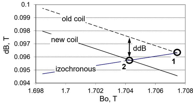
Figure 3: Changing of magnetic field level for operation mode  $A/Z = 3$  with new coil.
