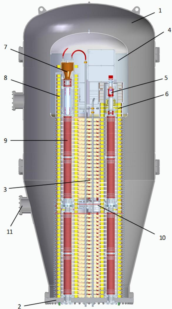
Figure 3: High voltage system of the electron cooler for NICA collider. 1 – pressure vessel, 2 – bottom flange, 3 – high voltage column, 4 – high voltage terminal, 5 – electron gun, 6 – gun solenoid, 7 – electron collector, 8 – collector solenoid, 9 – electrostatic tubes, 10 – middle section, 11 – side flange.
