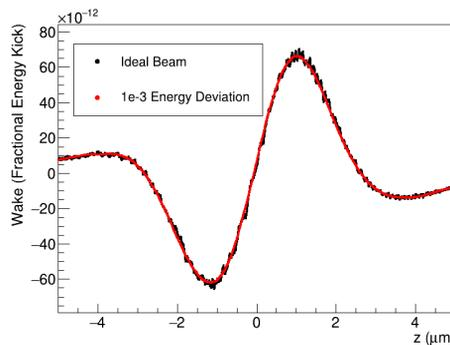
Figure 2: Comparison of the simulated wake at 275 GeV when we assume an on-energy electron beam and when the electron beam energy is offset by one part in 1000. No significant difference is present.
