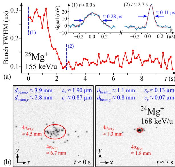
Figure 3: Electron cooling of slow, rf-bunched beams of  $Mg^+$ . Top (a): Evolution of the ion bunch length (15th harmonic) as a function of cooling time  $t$ . Bottom (b): Transverse beam sizes ( $d_{beam}$ ) and 95%-emittances ( $\epsilon$ ) before ( $t \approx 0$  s) and after ( $t \approx 7$  s) cooling, measured by imaging of neutral Mg atoms from charge-exchange (black dots).
