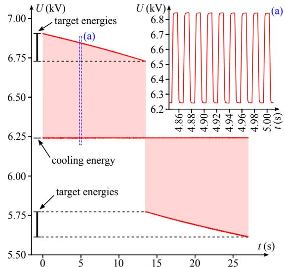
Figure 4: A typical ramp of the terminal voltage  $U$  during an experiment using the cooler as electron target. The inset (a) shows a magnified view of the 15-ms cycling between cooling and target energies, unresolved in the main plot.
