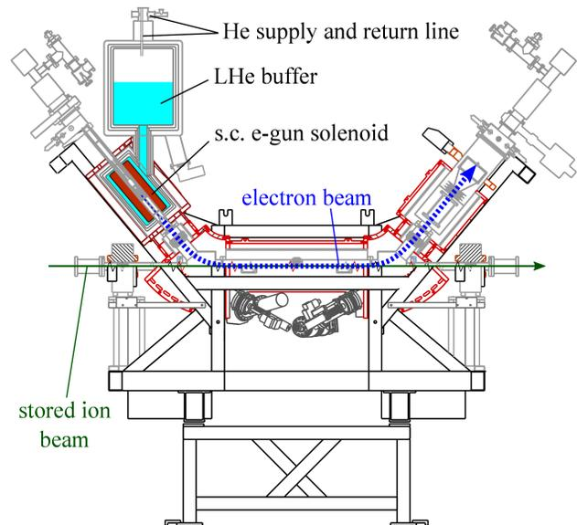
Figure 1: The CRYRING@ESR electron cooler.
