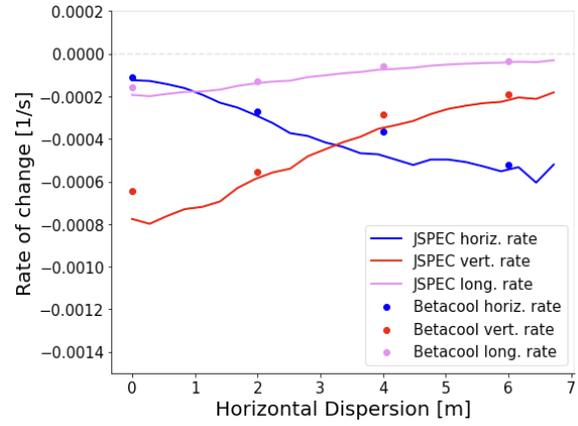
Figure 3: Comparison of JSPEC and Betacool for scans of horizontal dispersion and its effect on cooling rates.
