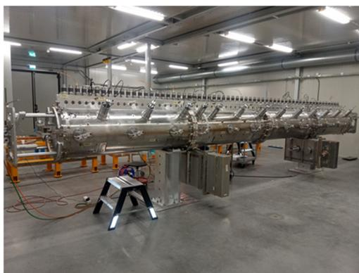
Figure 1: DTL1 on the bead pull station at ESS Lund.
