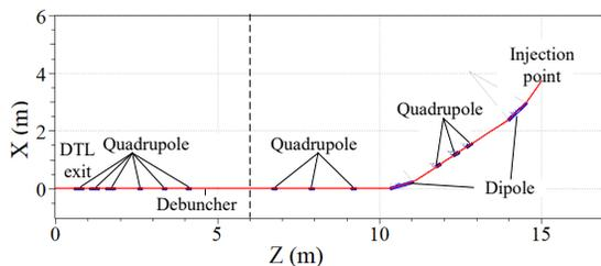
Figure 6: Layout of the main components of LRBT.
