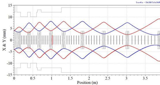
Figure 5: 2.45 times RMS beam envelope in the IH-DTL.
