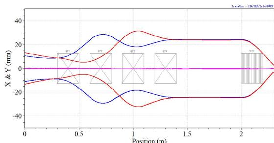
Figure 3: 2.45 times RMS beam envelope in the LEBT.
