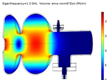
Figure 1: E-field distribution in the gun at  $E_{acc}=10\text{MV/m}$ .
