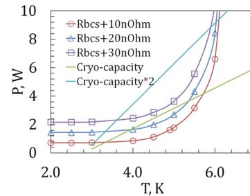
Figure 4: RF Power dissipation in the cavity at 10 MV/m and different temperatures together with the cryocooler capacity curve.
