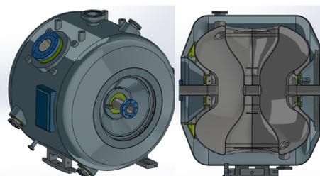
Figure 7: 3D model (on the left) and section view (on the right) of 325 MHz SSR2 dressed balloon cavity with EP ports.
