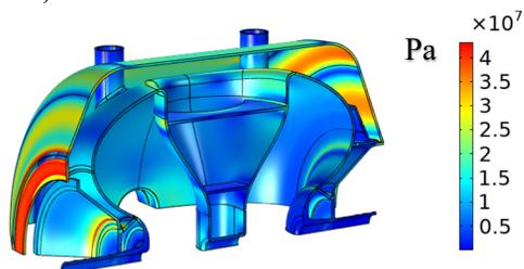
Figure 6: Stresses (Pa) in the dressed balloon cavity under 2.05 bar of He pressure.
