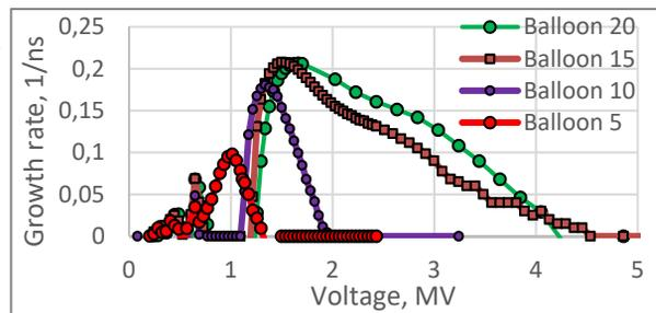
Figure 2: Balloon cavity multipactor (MP) performance for different spoke rounding.
