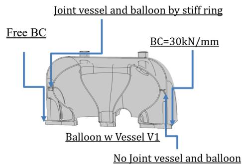
Figure 3: Dressed cavity model with helium vessel V1.
