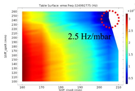
Figure 4: Frequency shift in the cavity with vessel V1 under 1 bar of external pressure.
