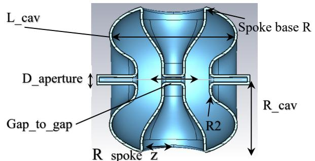
Figure 1: 325 MHz  $\beta = 0.475$  balloon cavity cross-section.
