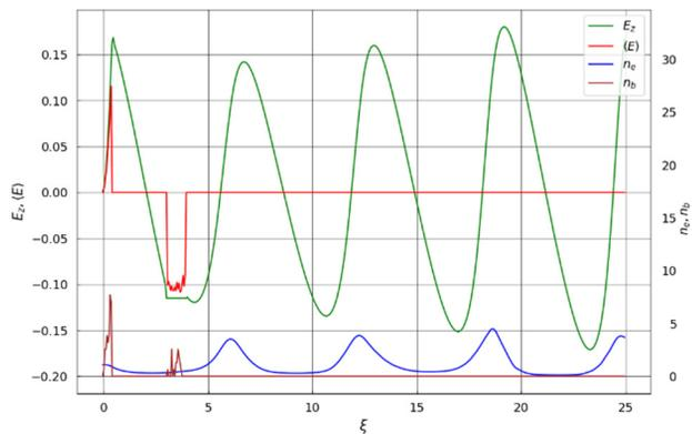
Figure 2: The on-axis wakefield excitation  $E_z$  by bunch-driver and plateau formation on  $E_z(\xi)$  by bunch-witness,  $\xi = z - V_b t$ . Densities of bunches  $n_b$  on the axis are shown by brown. Average field  $\langle E \rangle$  is shown by red. Plasma electron density is shown to be blue as a function of the coordinate  $\xi$  along the plasma. The parameters are the same as in Fig. 1. The maximum current of bunch-witness is equal to  $I_b = 0.7 \text{ kA}$ .
