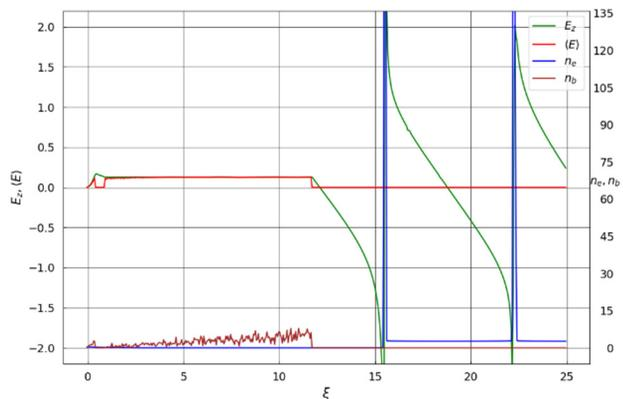
Figure 3: The on-axis wakefield excitation  $E_z$  by bunch-precursor and plateau formation on  $E_z(\xi)$  by bunch-driver,  $\xi = z - V_b t$ . Densities of bunches  $n_b$  on the axis are shown by brown. Plasma electron density is shown to be blue as a function of the coordinate  $\xi$  along the plasma. The parameters are the same as in Fig. 1. The maximum current of bunch-driver is equal to  $I_b = 11 \text{ kA}$ .
